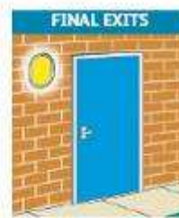
Install externally within 2 metres horizontal distance of any final exits. Please note that sufficient light will be needed to muster a roll call.
